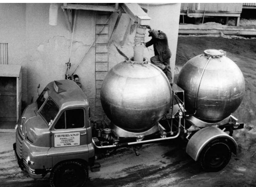
Donald Shepherd was full of innovative ideas. The portable silo was one of his most successful.
