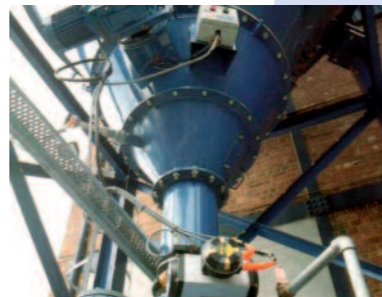
Portasilo's Rotoflo discharge unit and the Portasilo Superflow Dense Phase Conveying System.
